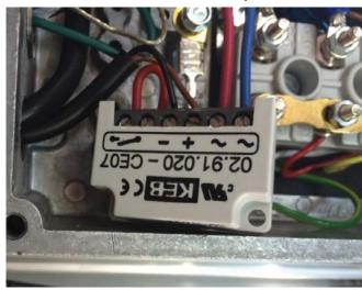
**Motor Connection** Black Motor White Cable Red Green Rectifier ⊕ **≀** ⊕ ≀ To Brake
